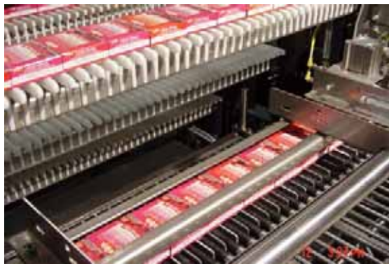
FIFO Accumulator with RWave® Transfer
